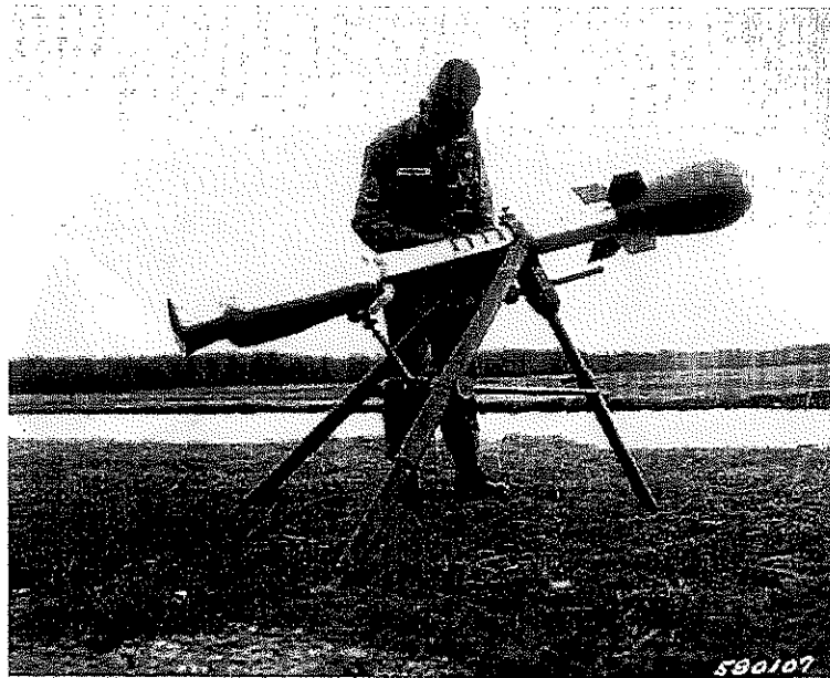
Figure 5.7 The Davy Crockett was the smallest and lightest nuclear weapon ever deployed by the U.S. military. It was designed for use in Europe against Soviet troop formations. ( http://en.wikipedia.org/wiki/File:DavyCrockettBomb.jpg )
