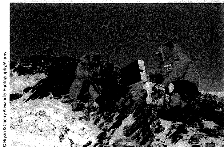
Figure 15.9 Research in Antarctica. Scientists set up a GPS receiver in west Antarctica as part of the west Antarctic GPS Network (WAGN) project. The WAGN project is measuring crustal movements surrounding the west Antarctic ice sheet. These movements in the lithosphere could affect the future of the ice sheet and its corresponding effect on sea level. How is this research related to global climate change?
