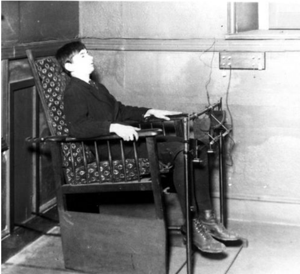
FIG. 2. This (circa 1903) photograph shows a young subject and the experimental apparatus Twitmyer used to measure the magnitude of the knee-jerk reflex (see http://www.psych.upenn.edu/history/twittext.htm for details).
