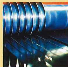
Slitting coils into finished strips.
