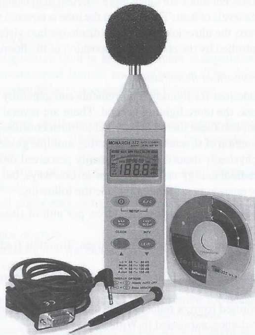
FIGURE 3.7 Weighted sound levels meters.
