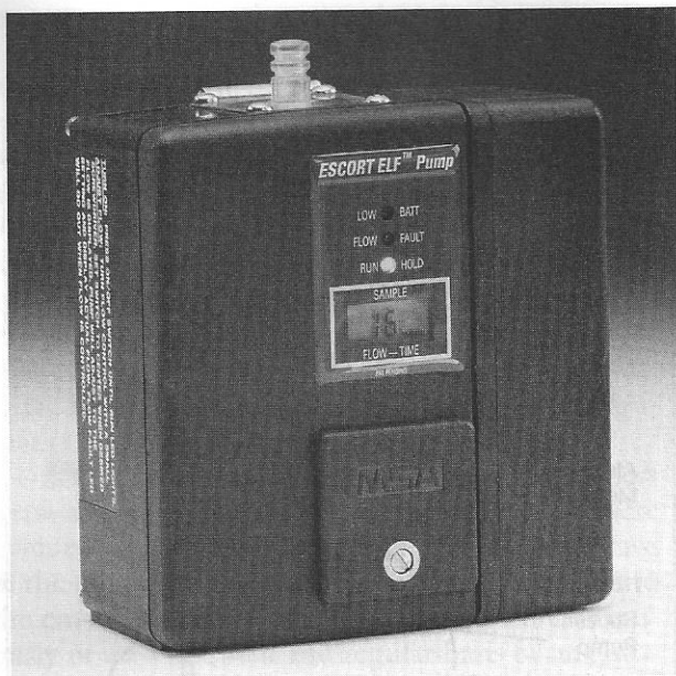
Figure 5-3: Personal sampling pumps such as this one are smaller and lighter than pumps commonly used for area sampling. Personal sampling pumps are used by the industrial hygienist to obtain data for evaluation against regulatory and other exposure limits.
