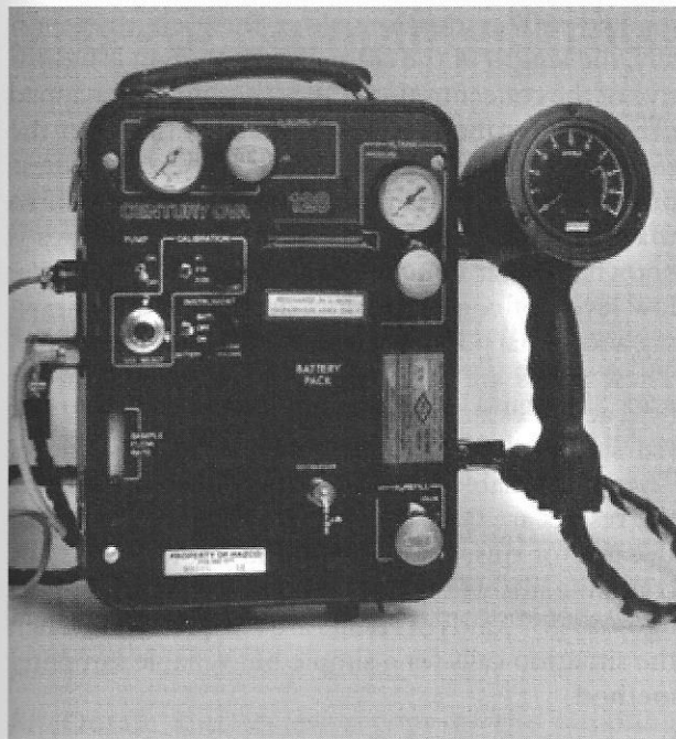
Figure 5-31: The flame ionization detector (FID) is another type of non-specific instrument often used at hazardous waste sites during investigation and cleanup. It is generally better than a PID at detecting hydrocarbon compounds, making them useful for field screening at sites where leaking underground fuel tanks have been removed.
