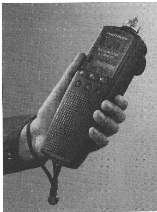
Figure 5-30: Photoionization detectors (PIDs) are direct-reading instruments that are used a great deal at hazardous waste sites. They are nonspecific, but useful for screening purposes during initial entries at sites where specific contaminants are unknown. The most common application is for screening to detect organic compounds.
