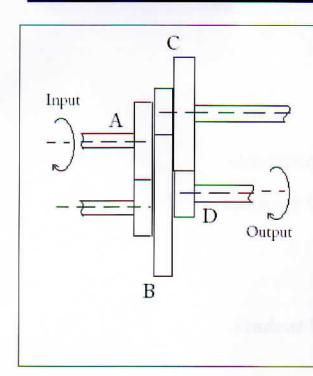
A and D are single spur gears
