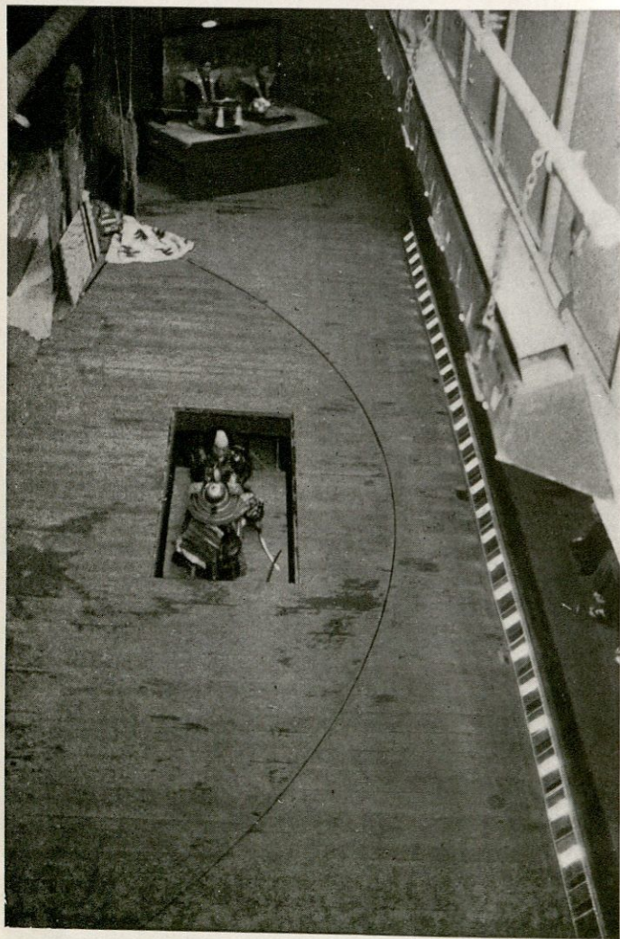
Two samurai enact a scene while rising on the "seriage." The curved line on stage shows a part of the revolving stage.
