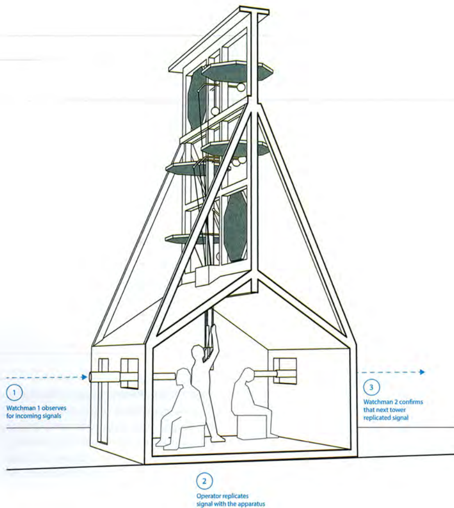
Diagram illustrating how the British shutter telegraph worked.
