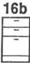
16b Drawer/file unit: two equal height drawers, one file drawer with compressor
