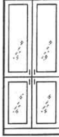
Two framed glass hinged doors above, two framed glass sliding doors below
