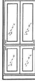
Two framed glass sliding doors above, two framed glass hinged doors below
