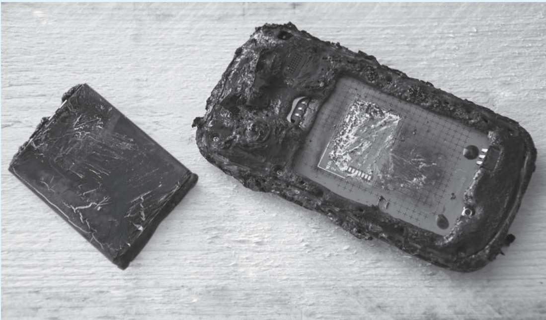
FIGURE 7.1 A Galaxy Note 7 Next to its Charred Battery after a Test
