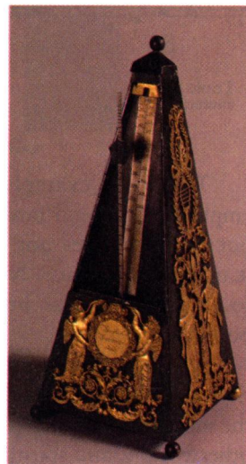
An early metronome owned by Beethoven; its inventor was a friend of his. A clockwork mechanism made the bar swing side to side, ticking at rates controlled by a movable weight.
