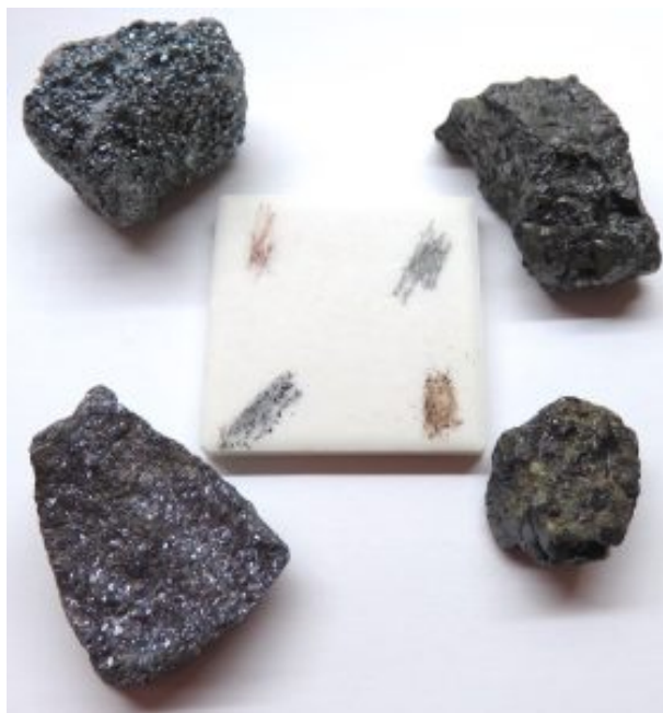
Figure 4.4 – Four different dark gray metallic minerals with varying streak colors. The minerals are from the upper left clockwise: hematite (red-brown), magnetite (black), sphalerite (honey-brown), and galena (dark gray). Image credit: Karla Panchuck , CC BY.
