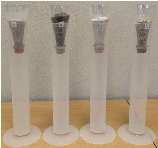
Figure 13.17 – Experimental set-up for various sediments to measure permeability. Image credit Chris Calvelage CC BY-NC-SA.
