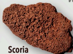
Figure 6.4 – Glassy and vesicular extrusive volcanic rocks. Obsidian is smooth with conchoidal fracture. Despite its dark color, it is felsic in composition. Scoria and pumice are highly vesicular. Scoria tends to be formed from basaltic magma, while pumice forms from felsic magma. Image credit: Karla Panchuk after Steven Earle; Photos by R. Weller/Cochise College, CC BY-NC-SA.
