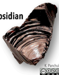
Figure 6.4 – Glassy and vesicular extrusive volcanic rocks. Obsidian is smooth with conchoidal fracture. Despite its dark color, it is felsic in composition. Scoria and pumice are highly vesicular. Scoria tends to be formed from basaltic magma, while pumice forms from felsic magma. Image credit: Karla Panchuk after Steven Earle; Photos by R. Weller/Cochise College, CC BY-NC-SA.
