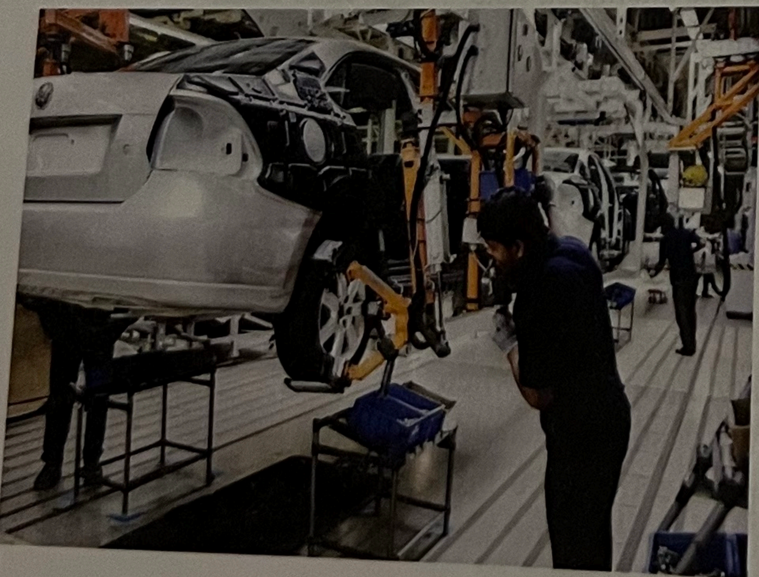
An employee uses a robotic arm to fit a wheel onto a Volkswagen AG Vento automobile on the production line at the Volkswagen India Pvt. plant in Chakan, Maharashtra, India.
