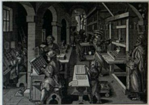
7. This Victorian engraving of a woodcut by Stradanus from about 1580 shows many stages of book production, including setting type, inking it, printing the sheets, and proof-reading
