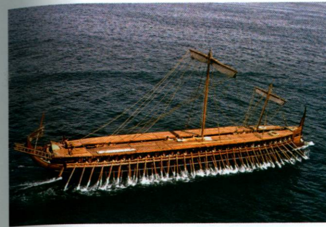
A MODERN REPLICA OF AN ATHENIAN TRIREME. These versatile warships were much more powerful than the old 50-oared pentakonters that had been in use for centuries. As the name suggests, a trireme featured three banks of oars on each side, 170 oars in total. These were manned by citizen rowers seated on benches at three different levels in the vessel’s hold. In battle, rowers could help power a ship forward, turn it, and keep it on course in a chase, even when sailing into the wind. In favorable winds, sails could be used to add speed. ■ How does this new military technology build on some of the same strategies as hoplite warfare?
