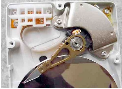
The mechanism that moves the arms on a hard disk has to be incredibly fast and precise. It can be constructed using a high-speed linear motor.
