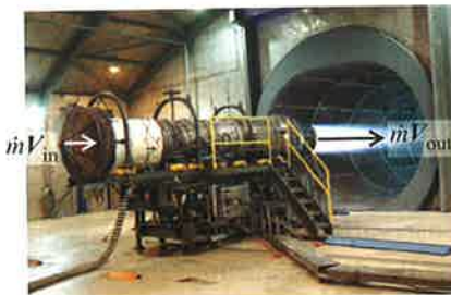
The horizontal reaction force exerted by the test stand on this jet engine equals the difference between the momentum flow out and the momentum flow in.
