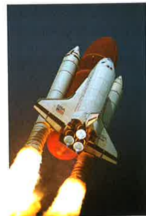
The momentum within a control volume defined by the exterior surfaces of the Space Shuttle changes as a result of two factors: the mass decreases as the propellants are consumed and expelled, and the velocity increases as the system accelerates.
