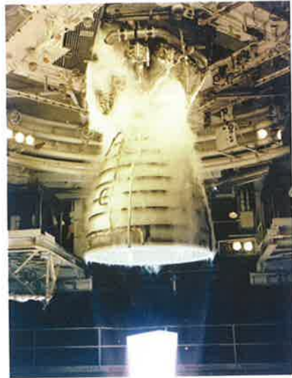
FIGURE 6.18 The Space Shuttle main engine secured in a test stand burns hydrogen with oxygen to create a high-velocity gas flow at the nozzle exit. Photograph courtesy of NASA.
