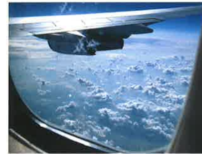
To maintain steady, level flight, the drag force is balanced by a net horizontal momentum flow from the aircraft's engines.
