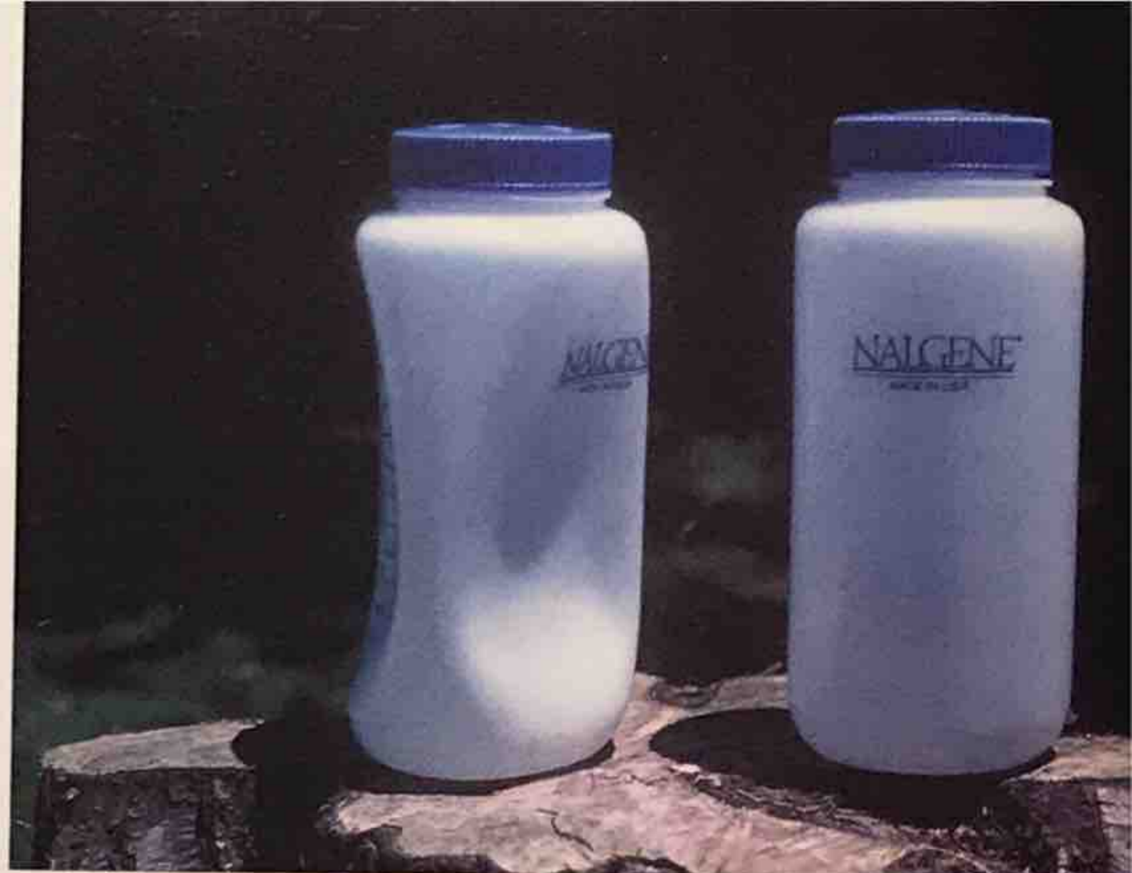
▲ Figure 5-2 The empty plastic bottle on the left was opened and then sealed tightly at an elevation of 3030 meters (9945 feet); when the bottle is brought down to sea level, the surrounding higher atmospheric pressure partially collapses the bottle. The bottle on the right contains air at sea-level pressure.
