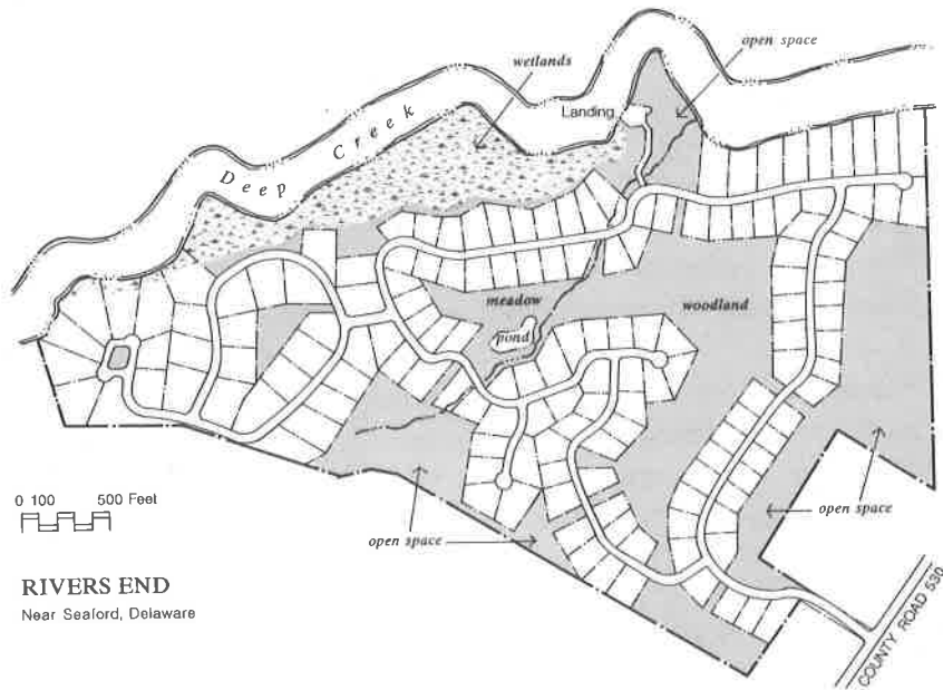
Figure 5-3. The site plan for River's End, near Seaford, Delaware, shows the relationship of its 142 lots to the 100 acres of open space preserved in this layout, including woodlands, meadows, ponds, streams, wetlands, riverbanks, and a neighborhood boat landing. Very few non-golf course developments in Delaware contain significant open space features such as these.
