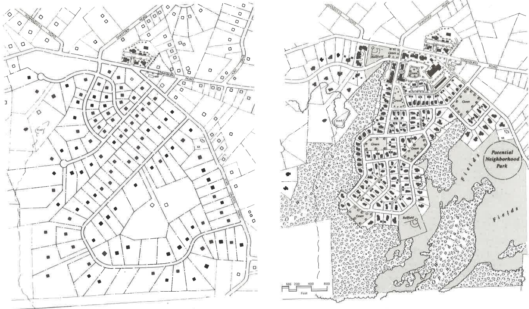
Figure 5-1. Site plan for the proposed expansion of Romansville, an historic hamlet within the rural/suburban township of West Bradford, Chester County, Pennsylvania. The author's design (at right) retains the entire density of the developer's original "cookie-cutter" plan (shown on the left) but arranges the development in a more compact village-like manner that preserves a substantial greenbelt of woodlands and farm fields around its perimeter. Due to their very compact nature, neo-traditional village layouts do not have the same high proportion of "view lots" that are commonly found in well-designed "conservation subdivisions." To compensate for this, the Romansville design includes five internal greens or commons (plus two ballfields), a relatively high number for a development of approximately 150 houselots.
