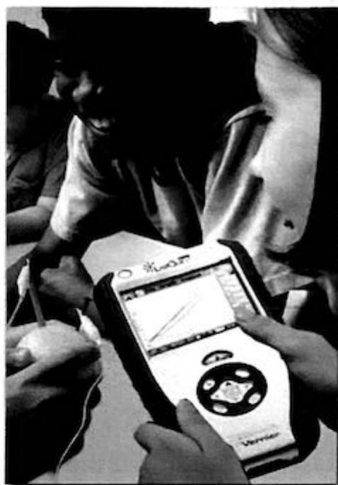
Figure 12.5 Sample Vernier LabQuest Probeware System
