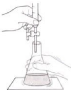
Figure 3 During a titration, the solution in the flask is swirled as NaOH is added to the acid sample.
