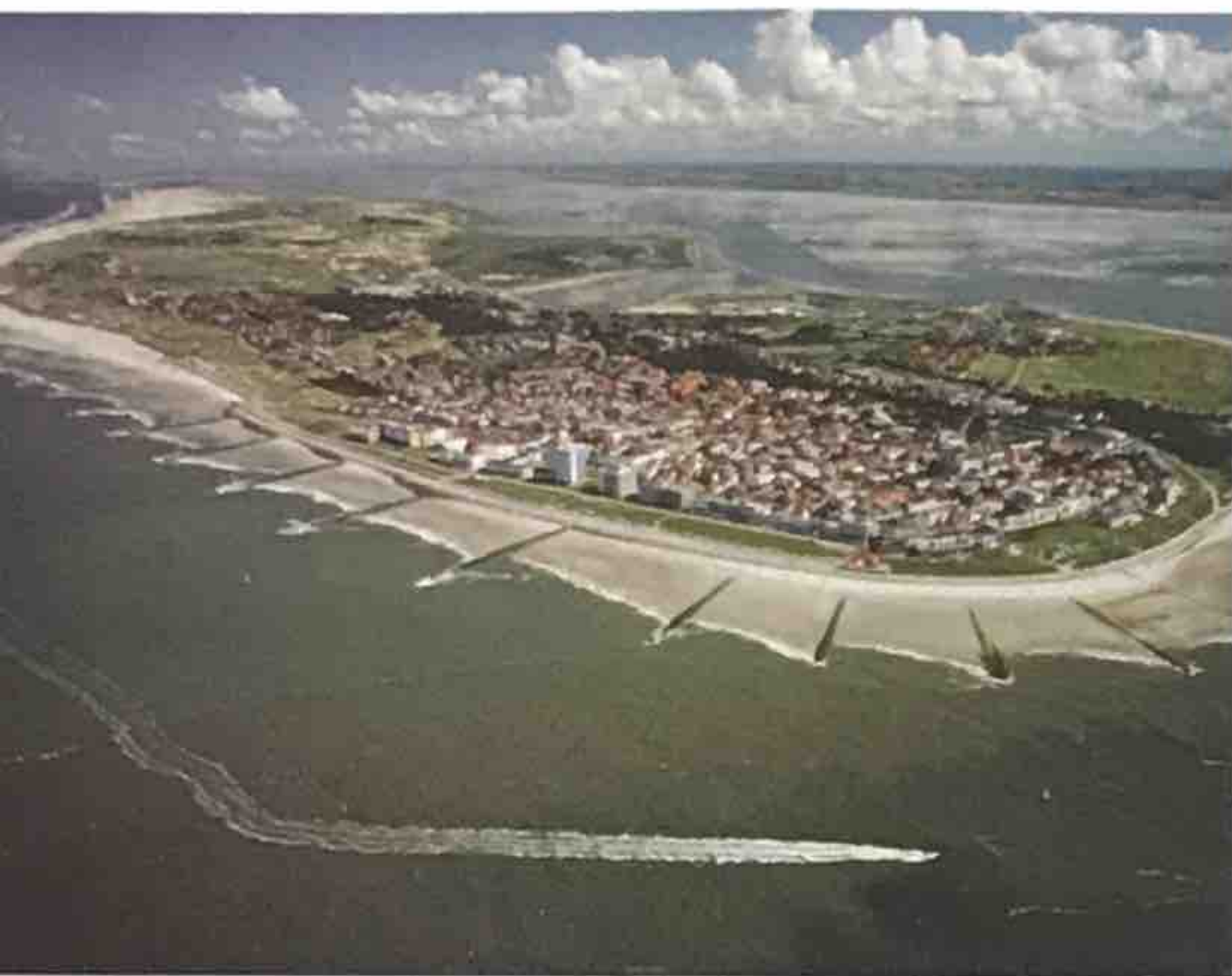
▲ Figure 20-26 Groin field along Norderney Island in northern Germany. The dominant direction of the longshore current is from left to right.
