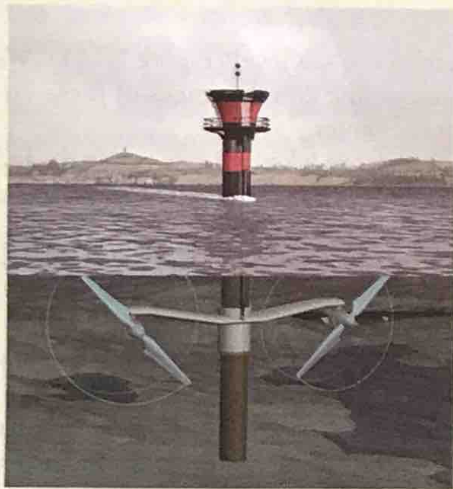
▲ Figure 20-D Tidal power turbines generate electric power when tidal currents turn underwater propellers that in turn power generators.
