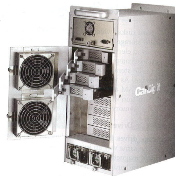
Figure 7-6 RAID storage device
