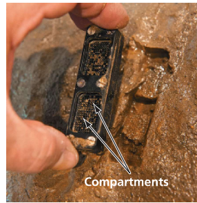
(b) A device used to grow potentially helpful species of bacteria in soil
