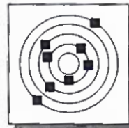
Polar Shows relationship between a variable and angle measured in degrees (cyclical trends, pollution source vs. wind direction, etc.).
