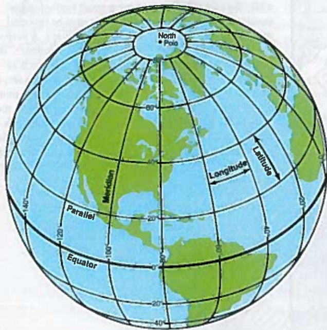
Figure 1.22 The grid system of parallels of latitude and meridians of longitude. Since the meridians converge at the poles, parallels become increasingly shorter away from the equator. On the globe, the 60th parallel (60°) is only one-half as long as the equator, and a degree of longitude along it measures only about 55 1/2 kilometers (about 34 1/2 miles) compared with about 111 kilometers (about 69 miles) at the equator (0°).
