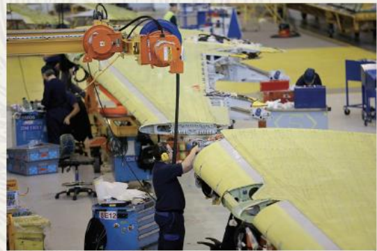
Wings are assembled at the Airbus SAS factory in Broughton, United Kingdom. Completed wings are transported to Toulouse, France, or Hamburg, Germany, for final assembly.
