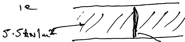
axles combined into one load known as knife edge load (KEL)
