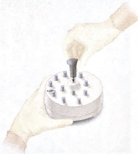
(2) Handle of dispenser is pushed down to place 12 disks on the medium. In addition to dispensing disks, this dispenser also tamps disks onto medium.
