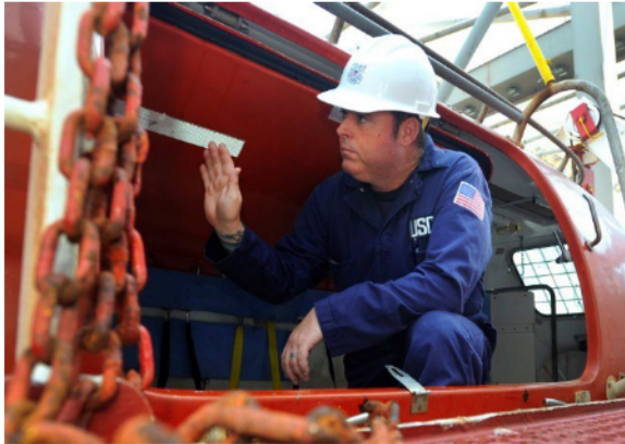
FIGURE 9 A USCG inspector inspects the life boat onboard a vessel. The inspection is part of a port state control examination, which is conducted periodically to ensure vessels are in compliance with safety regulations.
