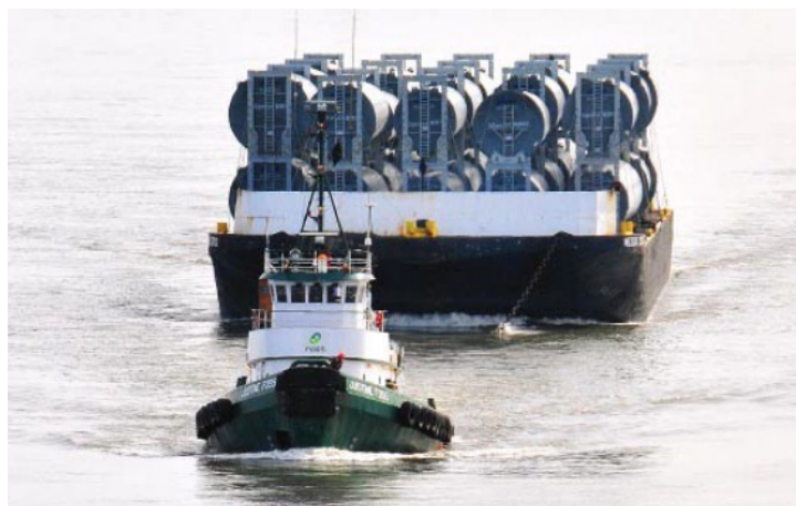
Figure 25 Barges can transport wind tower components via the MTS with greater ease than landside transportation due to the size and weight of the pieces.
